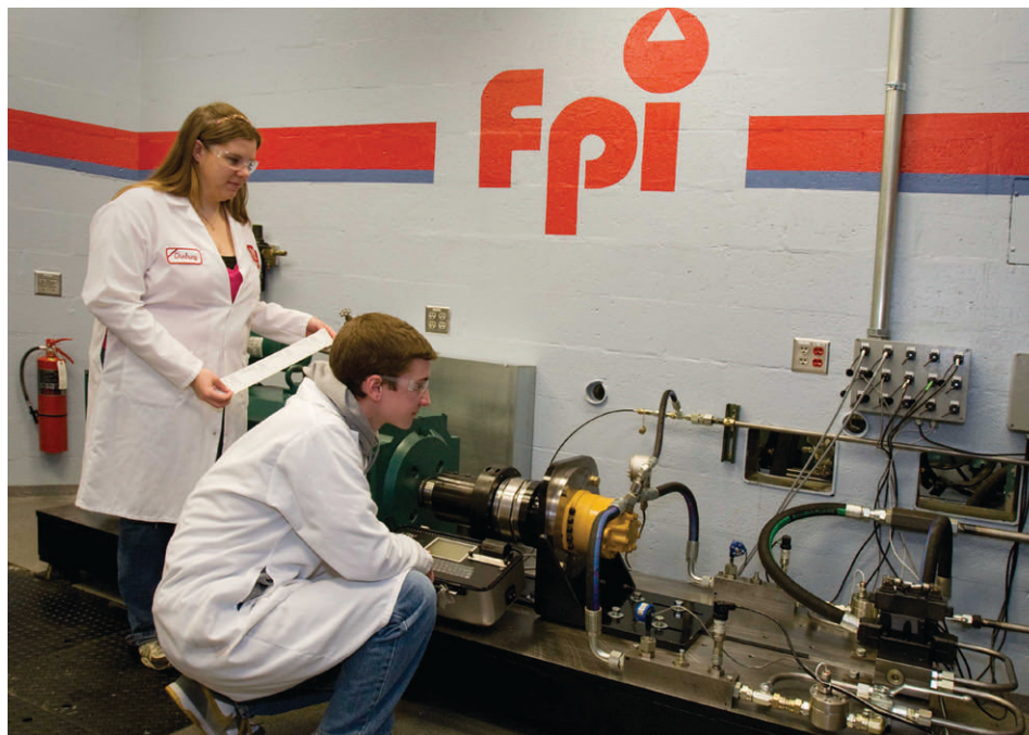
Milwaukee School of Engineering (MSOE) students Chelsey Jelinski and Brian Blazel examining the MSOE dynamometer used for efficiency testing of hydraulic motors.
